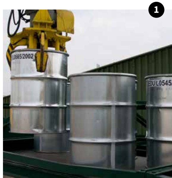
1 Once SÚRAO takes over responsibility for the waste drums, they are stacked on a rolling ramp. Provided the waste meets acceptability conditions, the drums are then moved to the pre-selected disposal chamber.
