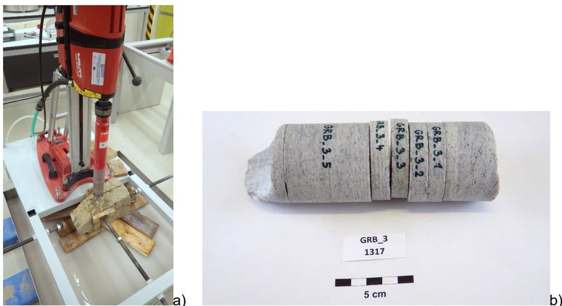
Fig. 2 a) Example of the drill-cutting of GRB (granulite) samples from a rock block, b) drill core samples following formatting for the laboratory analysis
