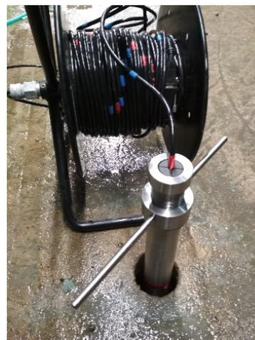
Fig. 62 Mechanical packer for a) borehole sealing b) sealing of the packer cable
