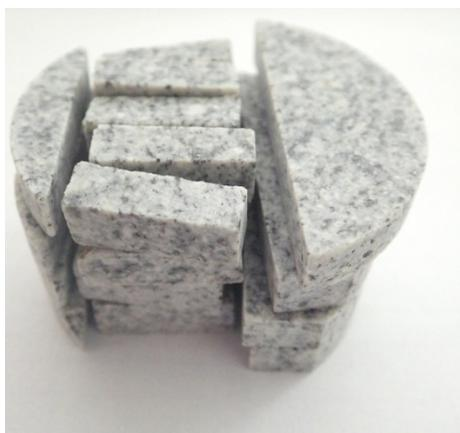
Fig. 14 Preparation of  $7 \times 7 \times 20$  mm samples for the study of the effective and Hg porosity of the D2 sample (Deštná) (50 mm)
