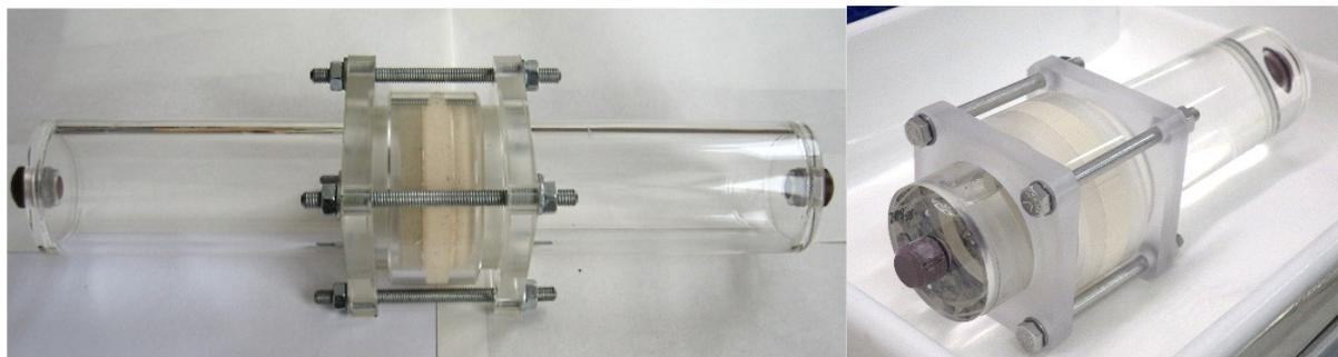
Fig. 51 Diffusion cell for the penetration diffusion experiments: ÚJV Řež design with various reservoir sizes
