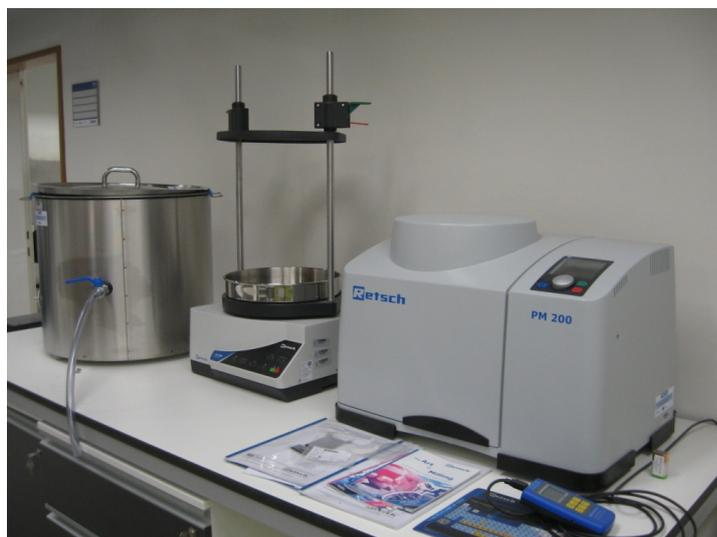
Fig. 4 PM 200 planetary ball mill (Retsch), AS 300 sieve shaker (Retsch) and a UV bath for sieve cleaning (description from right to left)
