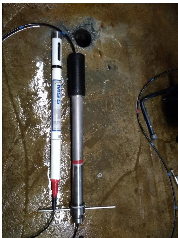
*Fig. 57 Minisonde 5 - MS5 fy OTT multiparametric probe, packer with cable bushing*
