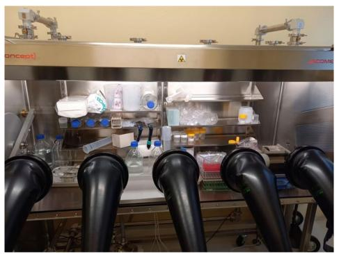
Fig. 7: Anaerobic glovebox with an inert argon atmosphere
