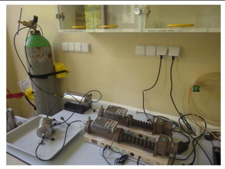
Fig. 6: Apparatus for the determination of the filtration coefficient K<sub>f</sub> at the ÚJV laboratory.
