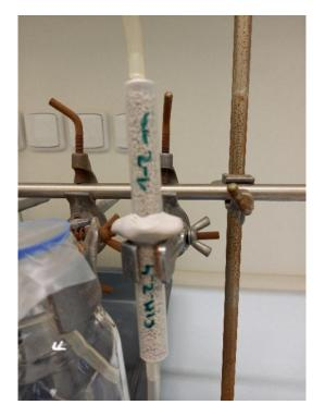
Fig. 9: Small column with the crushed cementitious material
